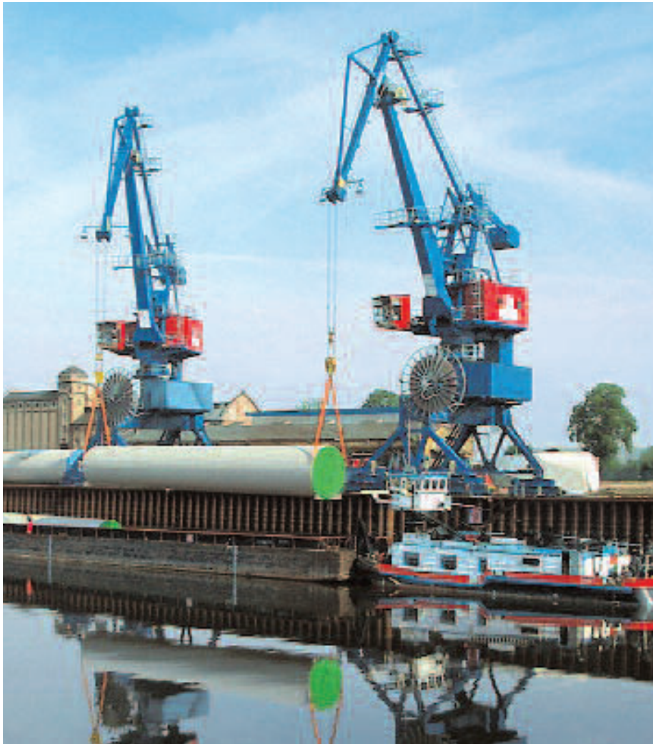
↑ Handling of parts of wind power plants by Tukan cranes
