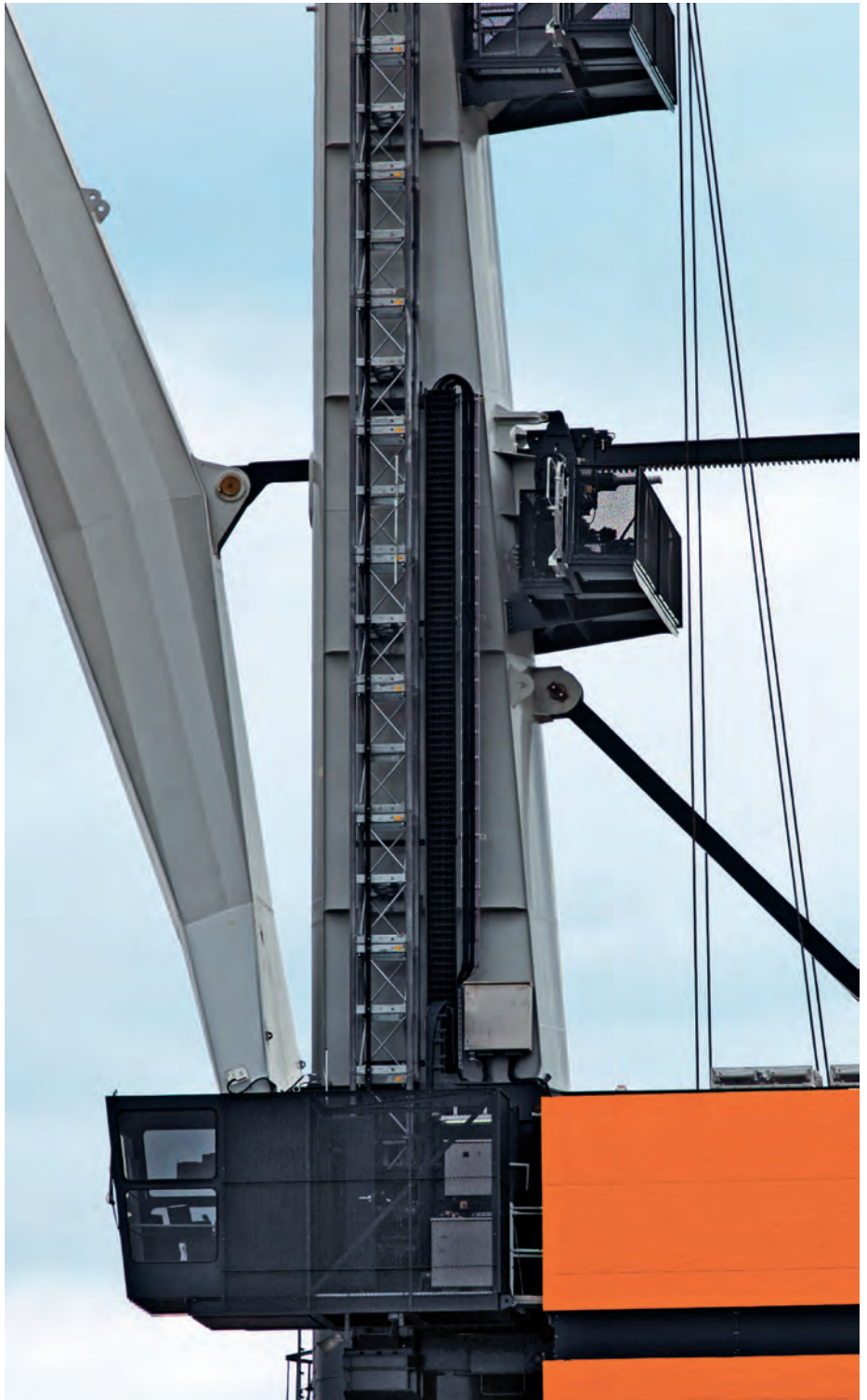
↑ Vertically adjustable driver's cab in the column
