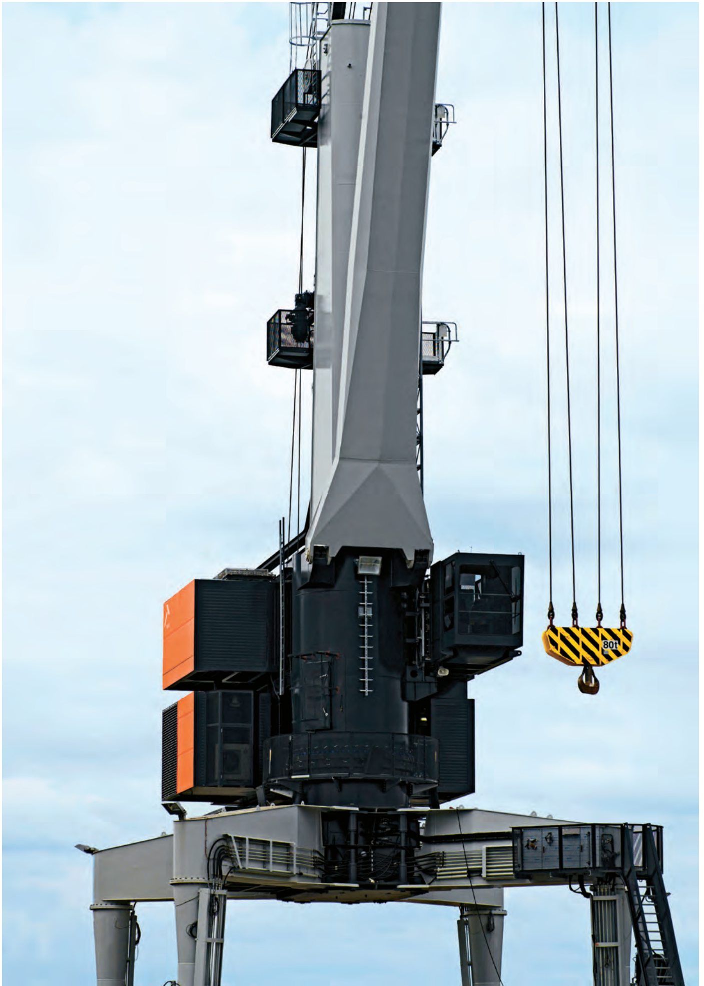
↑ The Adler – with a modular-design drive unit and vertically adjustable driver's cab
