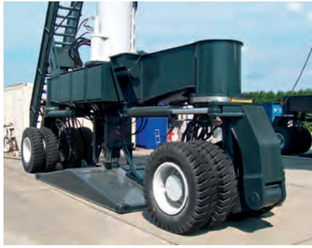
↑ Mobile travel mechanism with integrated propping system
