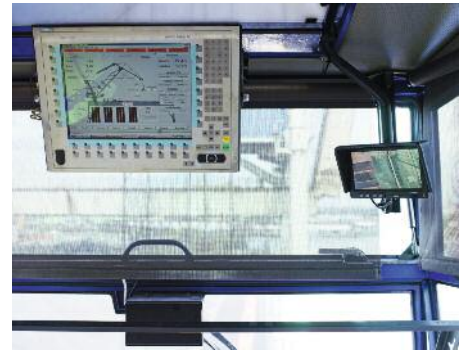
↑ Visualisation of crane data via the crane management system
