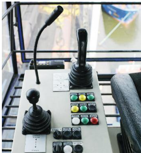
↑ Clearly arranged and ergonomically installed operating elements on the crane control stand
