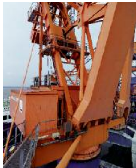
↑ Reliable and safe – rack and pinion luffing gears
